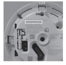
Place the device on the assembly plate with a slight anti-clockwise turn and then turn it clockwise without using too much force until it engages.
